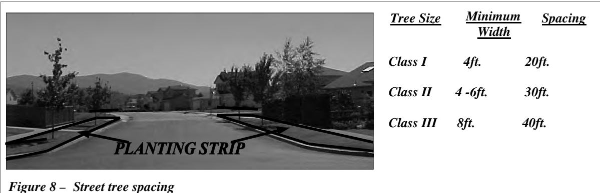
Figure 8 – Street tree spacing
